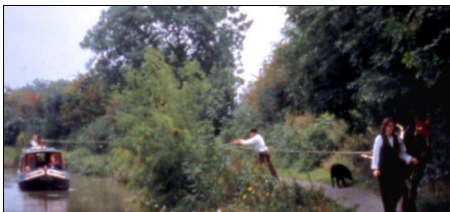
Branches that overhang the towing path from hedgerow bushes and trees are a hazard to horses, harness and pedestrians and need to be cut back to ensure that the full width of the towing path is clear at head height.
